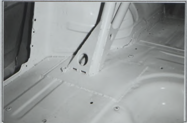
PHOTO No. 12 Rear upper rollbar to pillar
