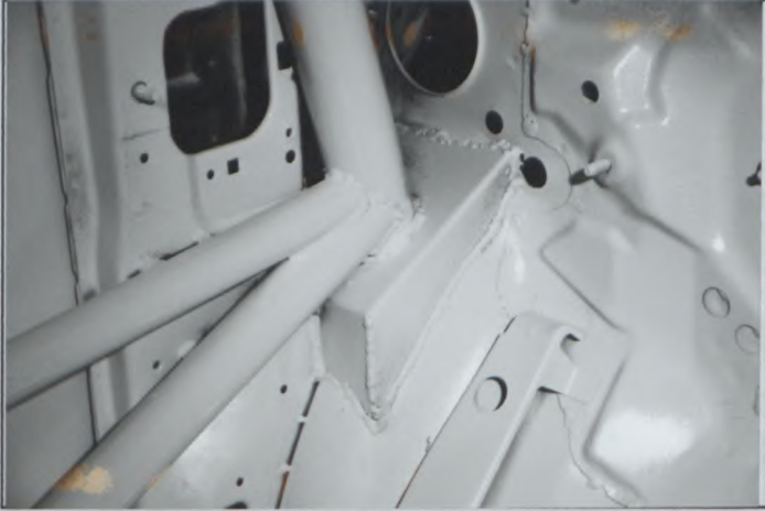
PHOTO No. 3 Front lateral rollbar to dash upper, center
