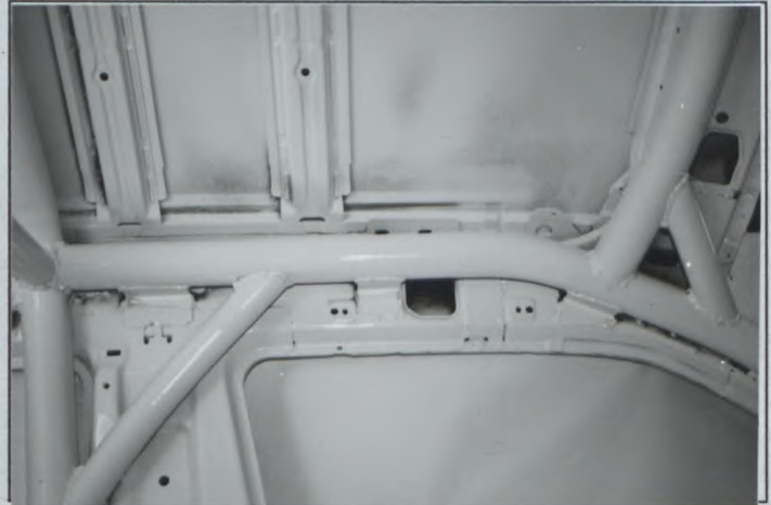
PHOTO No. 10 Rear support bars floor, rear
