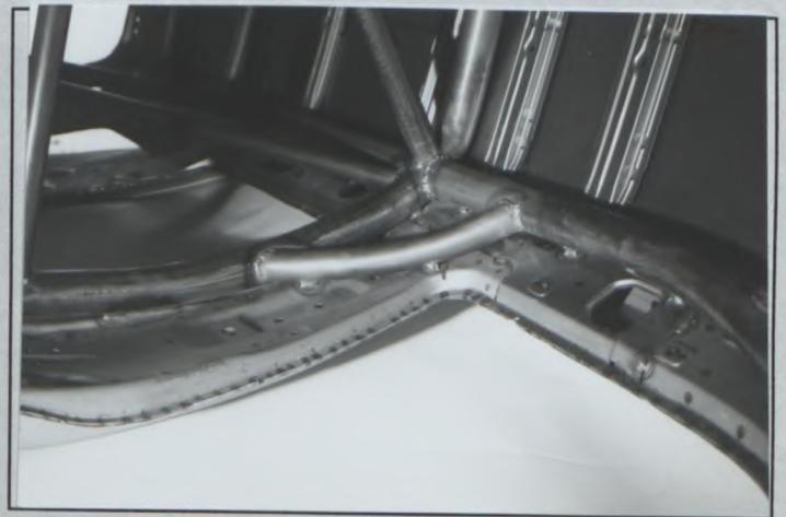
PHOTO No. 12 Front hoop to roof
