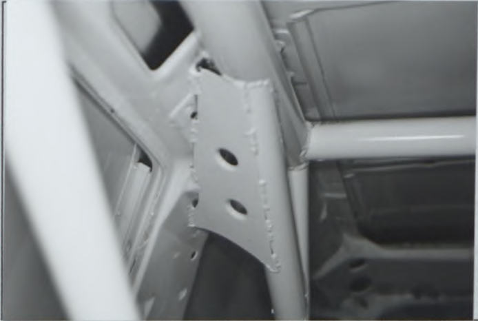
PHOTO No. 15 Front support bars to shock absorber tower
