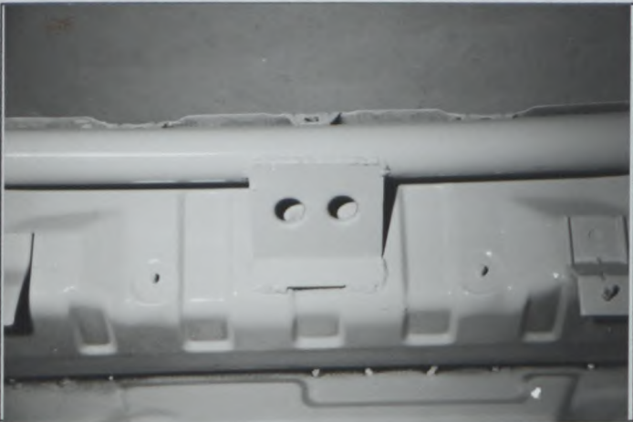
PHOTO No. 5 Longitudinal bar to floor
