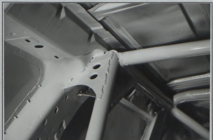
PHOTO No. 12 Rear upper rollbar to pillar
