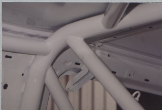
PHOTO No. 6 MAIN HOOP TO ROOF
