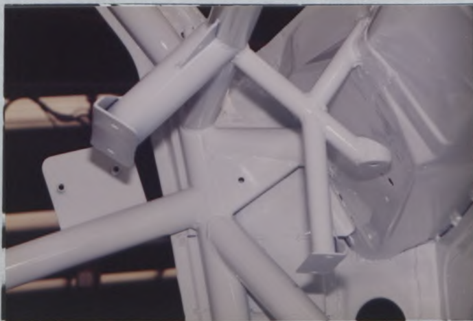
PHOTO No. 9 FRONT HOOP TO BULKHEAD
