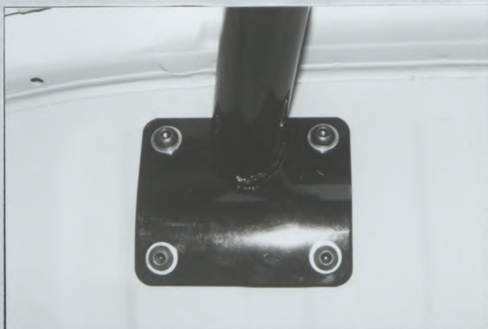
PHOTO N° 7. Rear support to wheel house LH
