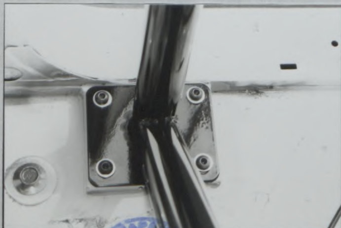
PHOTO N° 4. Main hoop to floor RH
