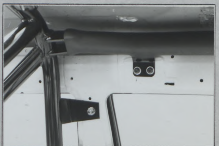
Main hoop to pillar
