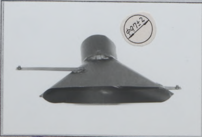
Photo Z5 Front brake cooling air intake TYPE C
