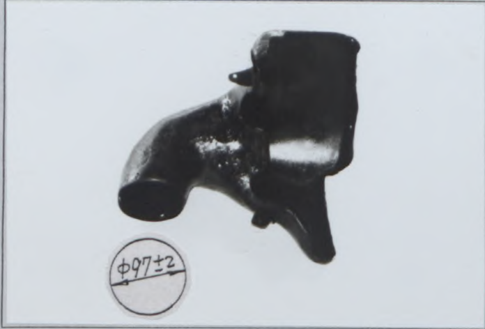
Photo Z1 Rear brake cooling air outlet TYPE C
