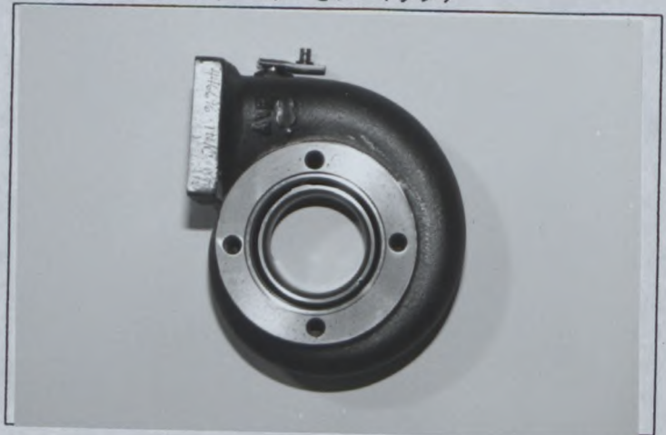
N) Turbine housing of turbocharger
