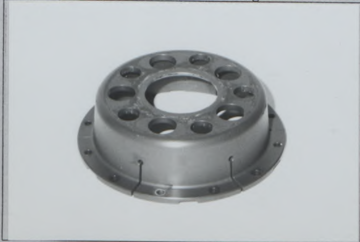
Photo W3 Rear brake mounting bell TYPE A
