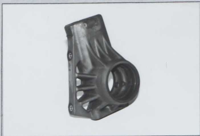
Photo T1 Front reinforced knuckle TYPE C
