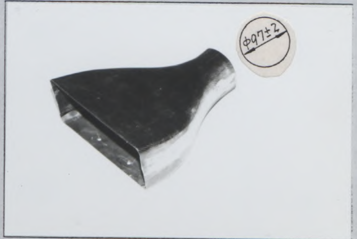
Photo Z6 Front brake cooling air intake TYPE D
