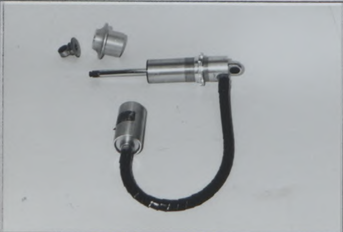
Photo TU11 Heavy duty front and rear shock absorber
