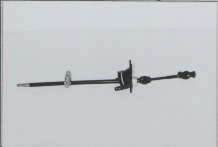
Photo Z12 Reinforced steering column
