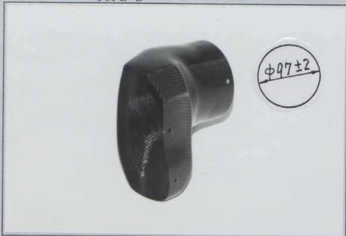
Photo Z5 Reinforced front differential casing TYPE B
