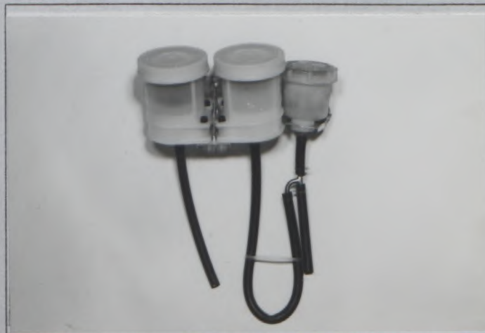
Photo Z3 Twin brake master cylinder reservoir tank
