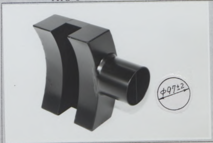
Photo Z4 Front brake cooling air outlet TYPE C
