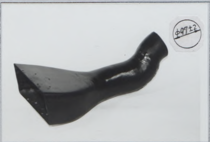
Photo Z1 Front brake cooling air intake TYPE G
