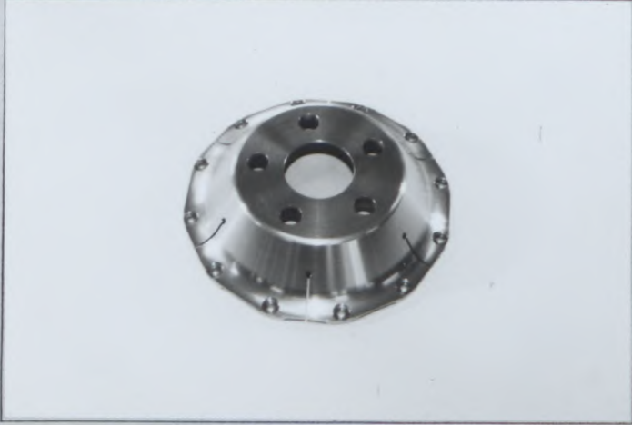
Photo V1 Front brake mounting bell TYPE G
