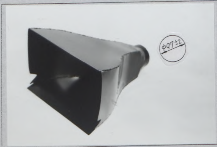
Photo Z3 Front brake cooling air intake TYPE F
