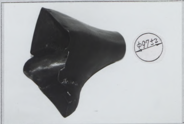
Photo Z4 Front brake cooling air outlet TYPE C
