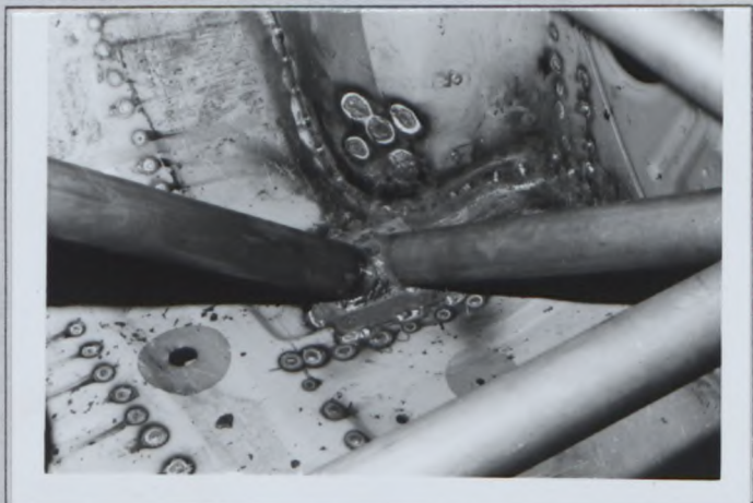
Rear left hand stay and main diagonal rollbar to floor
