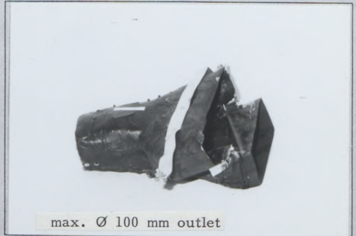
Photo Z9 Front brake cooling air intake
