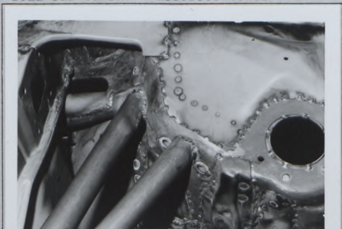
Front support bars and front lateral roll bar to shock absorber tower
