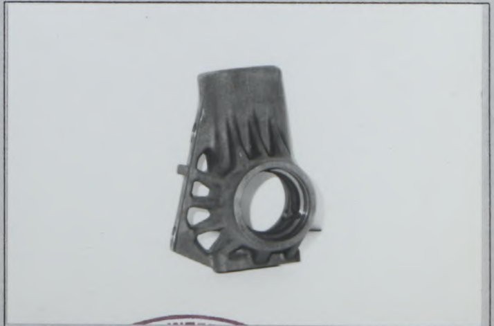
Photo T6 Reinforced knuckle TYPE B
