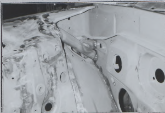
Front support bars to shock absorber tower
