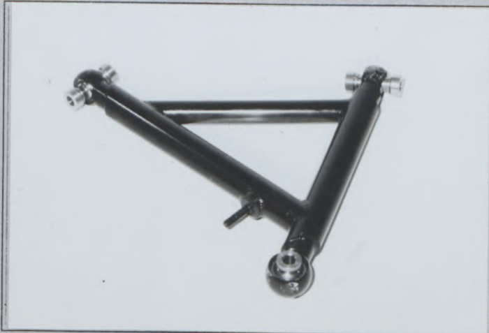
Adjustable rear stabilizer TYPE A with linkage
