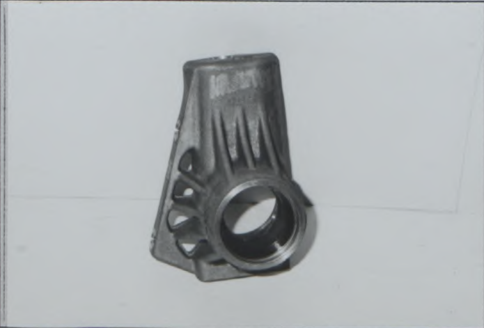
Photo T5 Reinforced knuckle TYPE A
