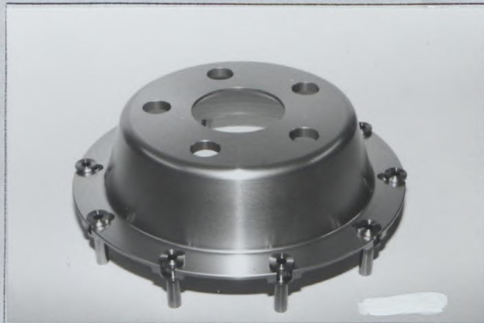
Photo Z2 Front brake cooling air intake TYPE H
