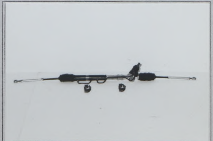
Photo Z13 Heavy duty steering gear box and side rods
