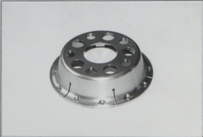
Photo VW6 Front and/or rear brake mounting bell TYPE J
