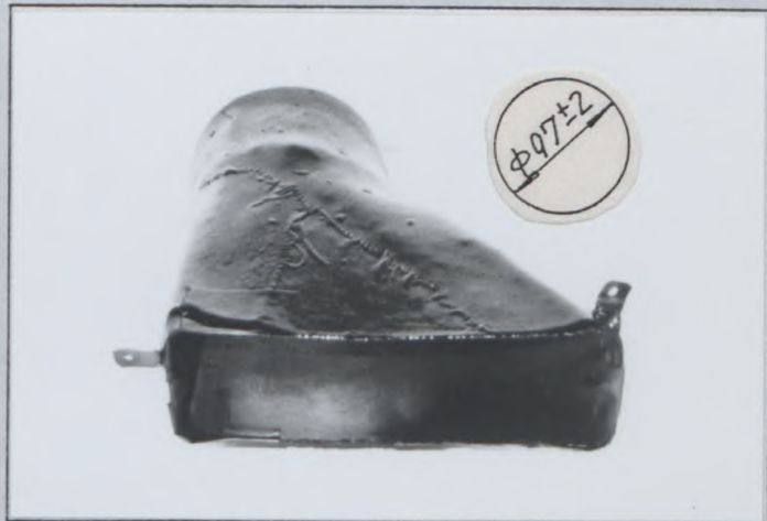
Photo Z8 Rear brake cooling air intake TYPE A
