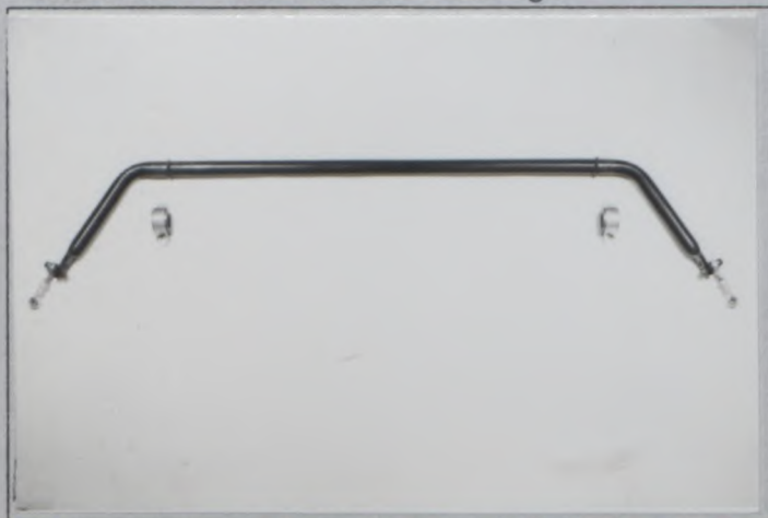
Photo U2 Adjustable rear stabilizer TYPE B with linkage
