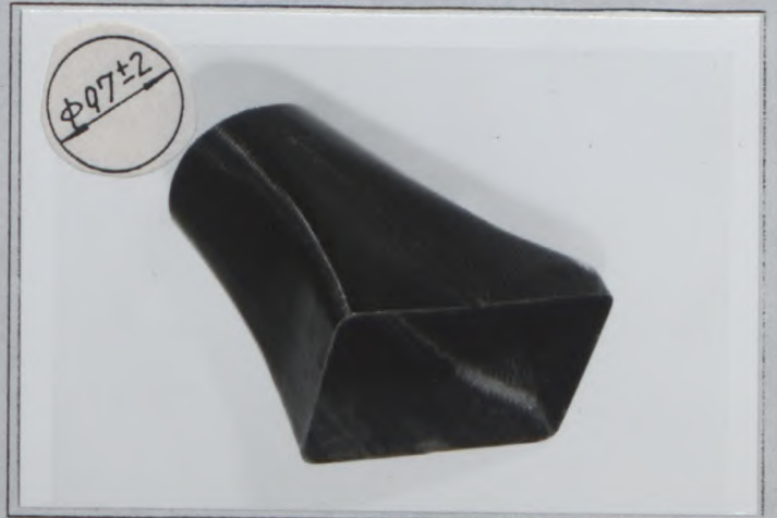
Photo Z6 Front brake cooling air intake TYPE D
