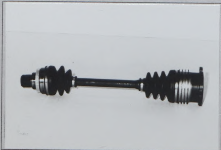
Photo Z6 Reinforced front left hand drive shaft
