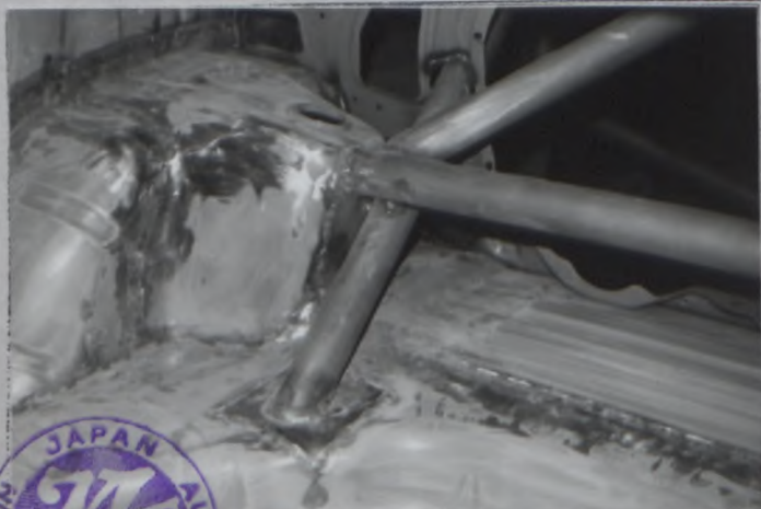
Rear left hand support to floor, rear diagonal rollbar and rear lateral rollbar to shock absorber tower
