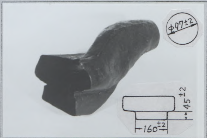
Photo Z2 Front brake cooling air intake TYPE H
