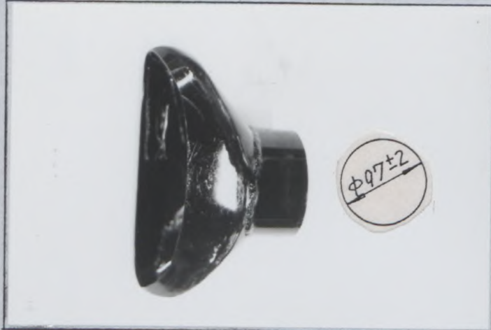
Photo Z7 Front brake cooling air outlet TYPE B
