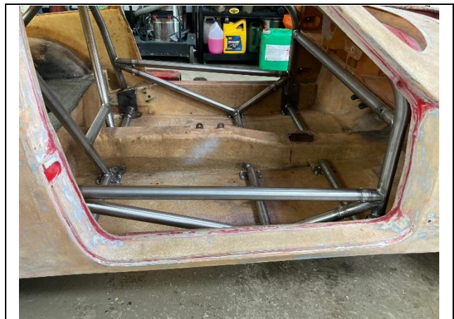
PHOTO 11 ANTI-INTRUSION DOORBAR – CO-DRIVER
