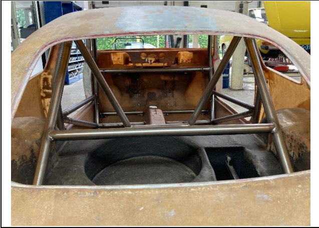
PHOTO 12 SHOULDER HARNESS ATTACHMENT – DRIVER
