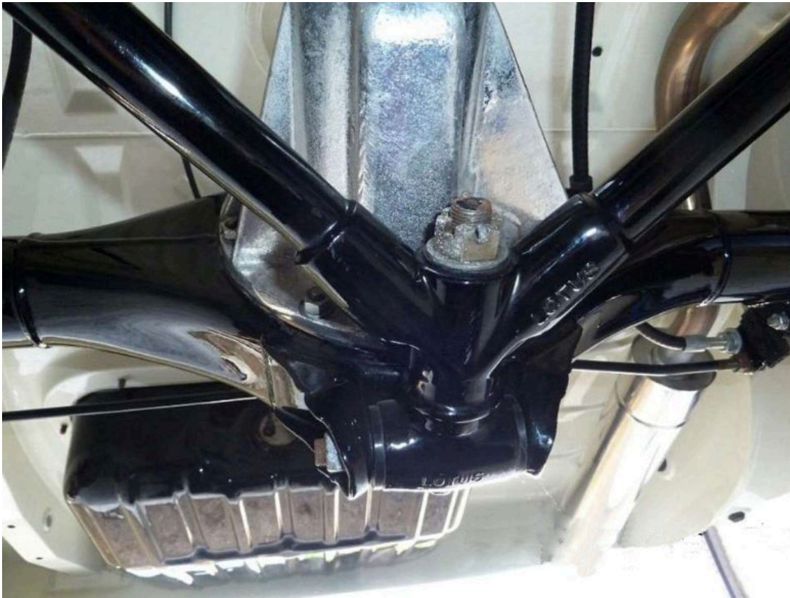
A Frame to differential mounting
