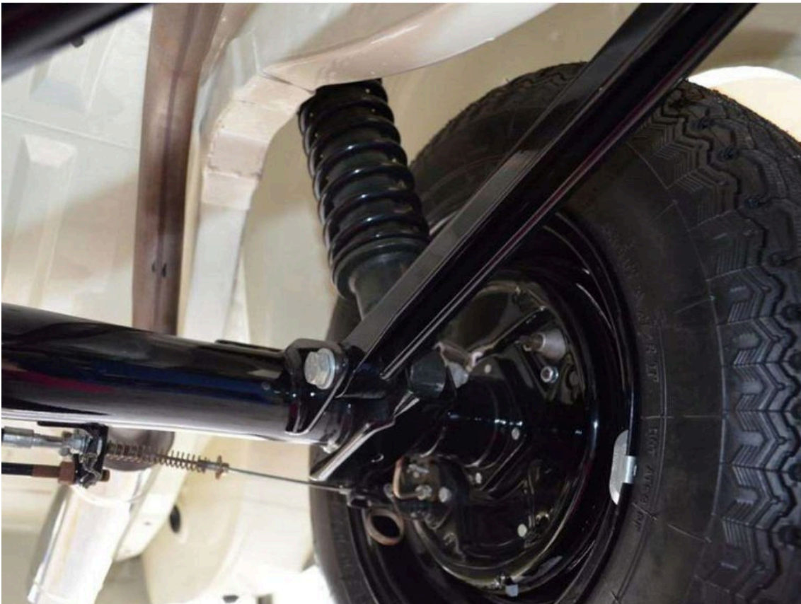
A Frame to differential mounting
