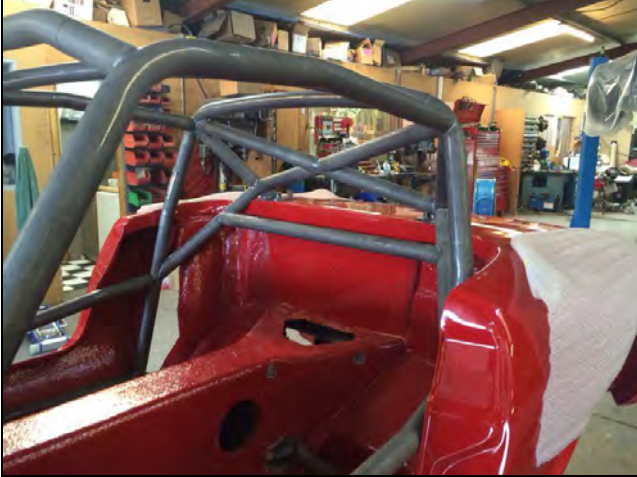
PHOTO 7 FRONT ROLLBAR ATTACHMENT TO "A" PILLAR
