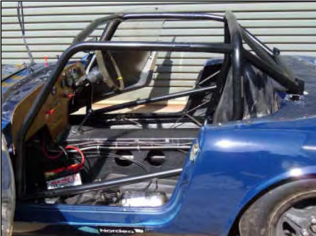
PHOTO 5 REAR BACKSTAY TO BODY ATTACHMENT
