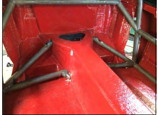
PHOTO 8 MAIN ROLLBAR ATTACHMENT TO "B" PILLAR
