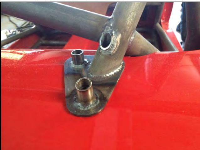
PHOTO 5 REAR BACKSTAY TO BODY ATTACHMENT
