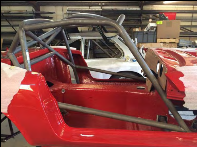
PHOTO 5 REAR BACKSTAY TO BODY ATTACHMENT
