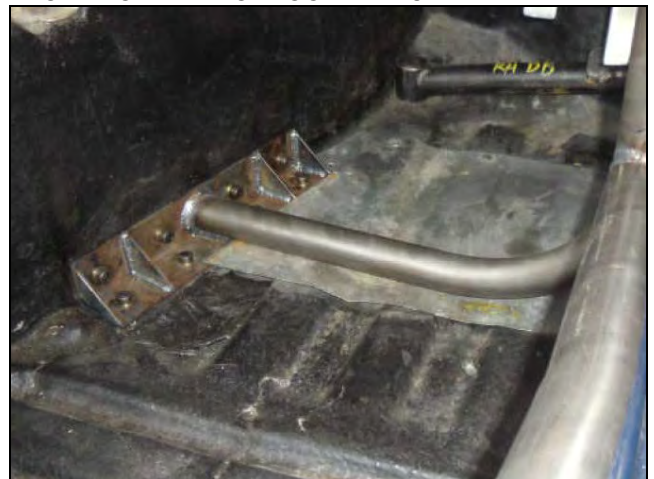
PHOTO 6 FRONT ROLLBAR TO FLOOR ATTACHMENT
