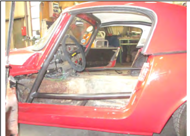
PHOTO 5 REAR BACKSTAY TO BODY SHELL ATTACHMENT
