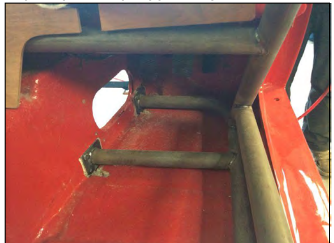
PHOTO 6 FRONT ROLLBAR TO FLOOR ATTACHMENT
