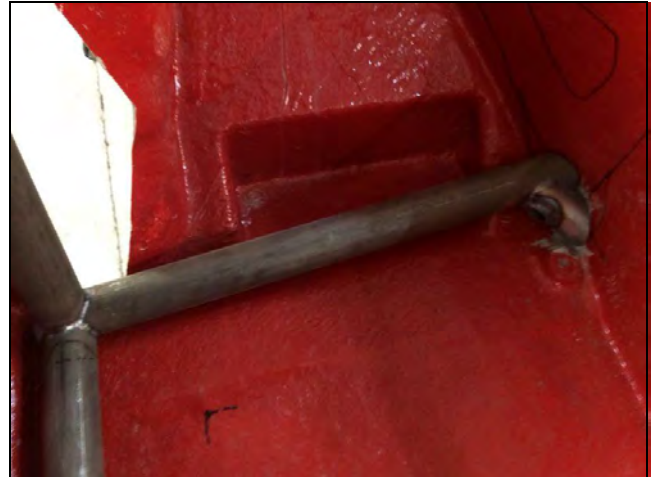
PHOTO 6 FRONT ROLLBAR TO FLOOR ATTACHMENT
