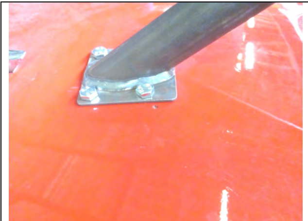
PHOTO 5 REAR BACKSTAY TO BODY SHELL ATTACHMENT
