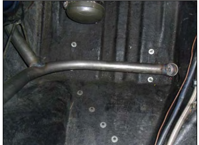
PHOTO 6 FRONT ROLLBAR TO FLOOR ATTACHMENT
