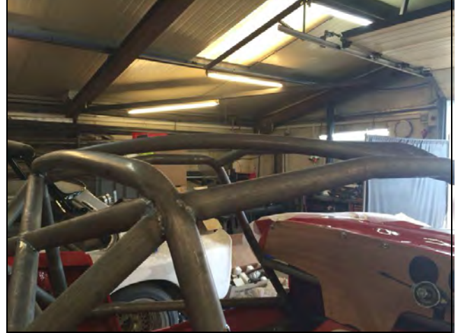
PHOTO 4 MAIN ROLLBAR TO FLOOR ATTACHMENT
