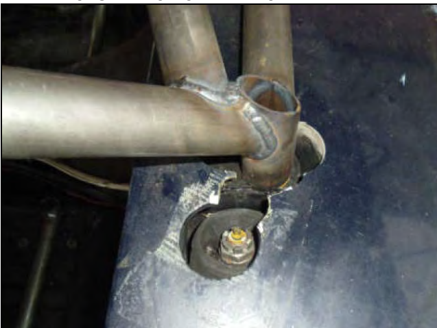
PHOTO 5 REAR BACKSTAY TO BODY ATTACHMENT
