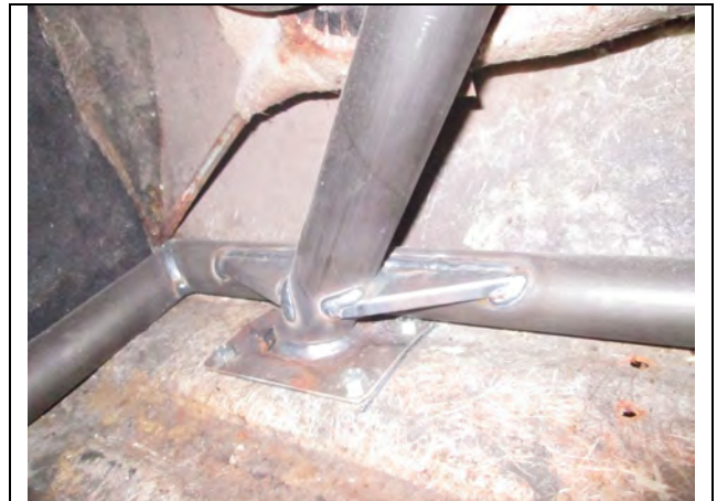
PHOTO 6 FRONT ROLLBAR TO FLOOR ATTACHMENT
