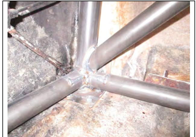
PHOTO 6 FRONT ROLLBAR TO FLOOR ATTACHMENT
