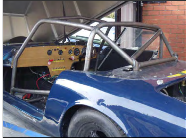
PHOTO 4 MAIN ROLLBAR TO FLOOR ATTACHMENT
