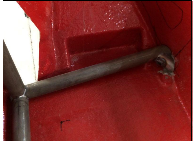
PHOTO 6 FRONT ROLLBAR TO FLOOR ATTACHMENT
