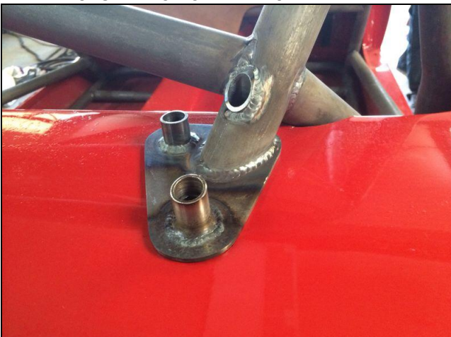
PHOTO 5 REAR BACKSTAY TO BODY ATTACHMENT
