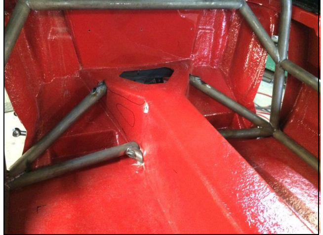
PHOTO 8 MAIN ROLLBAR ATTACHMENT TO "B" PILLAR
