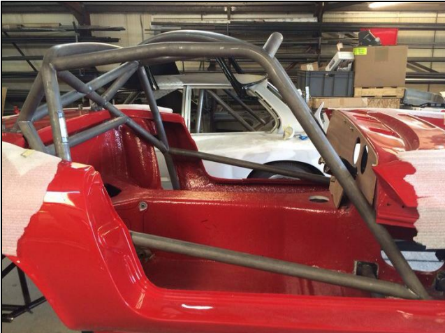
PHOTO 5 REAR BACKSTAY TO BODY ATTACHMENT
