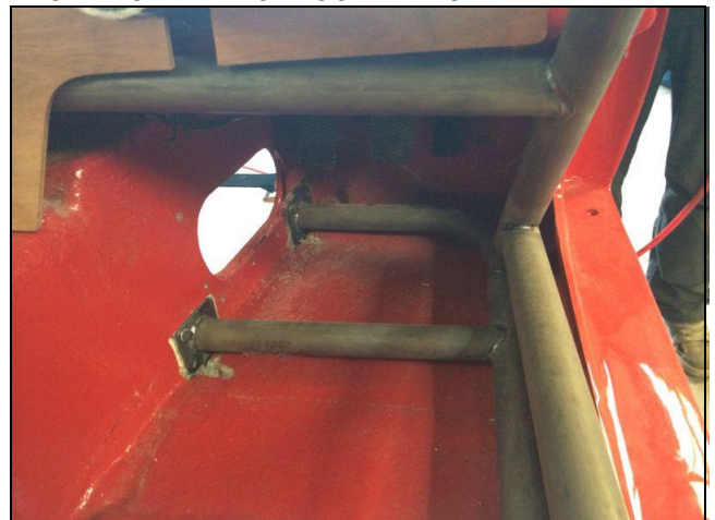
PHOTO 6 FRONT ROLLBAR TO FLOOR ATTACHMENT
