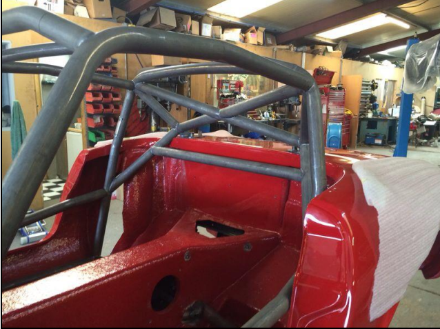
PHOTO 7 FRONT ROLLBAR ATTACHMENT TO "A" PILLAR
