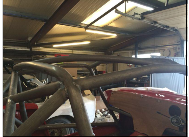
PHOTO 4 MAIN ROLLBAR TO FLOOR ATTACHMENT
