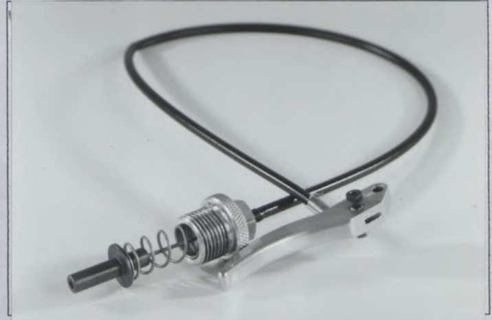
PHOTO No S2 Additional gearbox reverse gear control linkage
