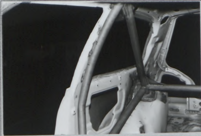
Main hoop to pillar
