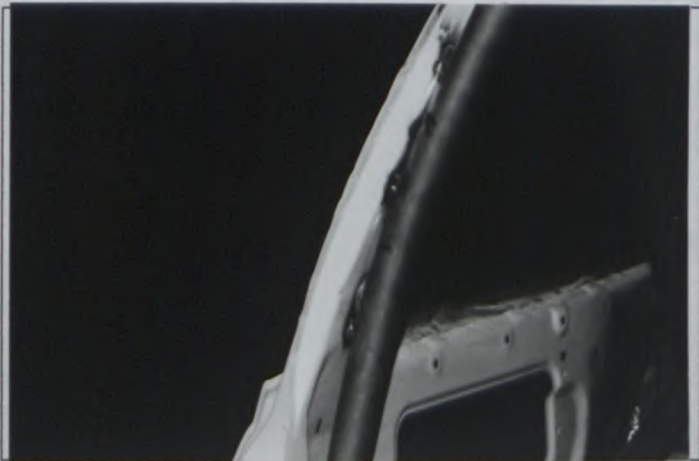
Main hoop to pillar
