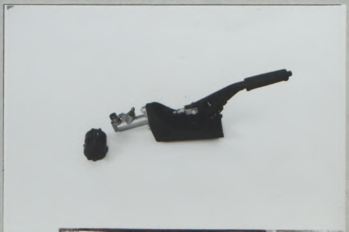
PHOTO NO. 12 (PARKING BRAKE)
