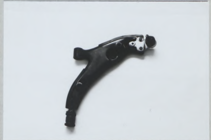
PHOTO NO. 2 (REINFORCED LOWER ARM : TYPE B)
