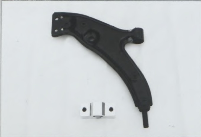
PHOTO NO. 1 (REINFORCED LOWER ARM : TYPE A)
