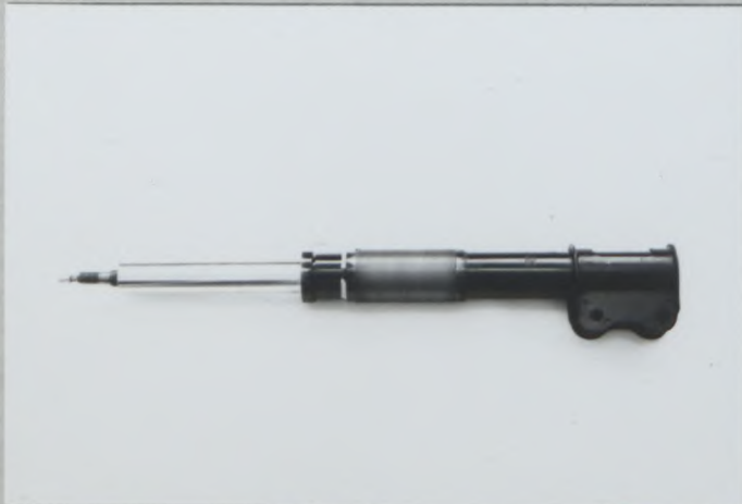
PHOTO NO. 3 (REINFORCED FRONT STRUT)
