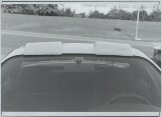
PHOTO 1 4 : FLAPS FOR VENTILATION TYPE 2
