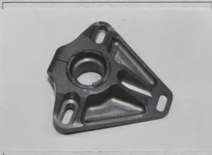
PHOTO 31 FRONT REINFORCED TOP MOUNTING PLATES
