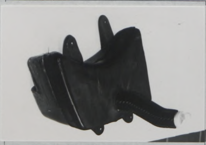
PHOTO 123 WATER TANK INCLUDING ELECTRIC PUMP FOR BRAKE AND/OR SHOCK ABSORBER COOLING
