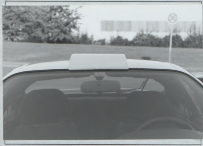
PHOTO 1 3 : FLAPS FOR VENTILATION TYPE 1
