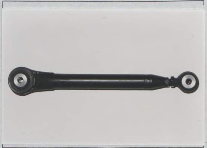
PHOTO 44 REINFORCED FRONT CROSS TIEROD OF THE REAR SUSPENSION TYPE B
