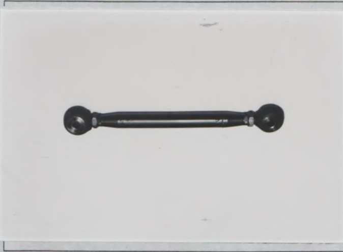
PHOTO 43 REINFORCED FRONT CROSS TIEROD OF THE REAR SUSPENSION TYPE A
