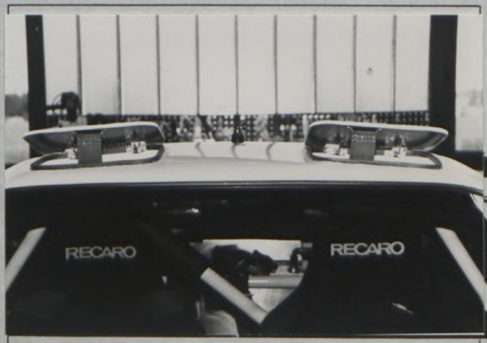
PHOTO 120 FLAPS FOR VENTILATION
