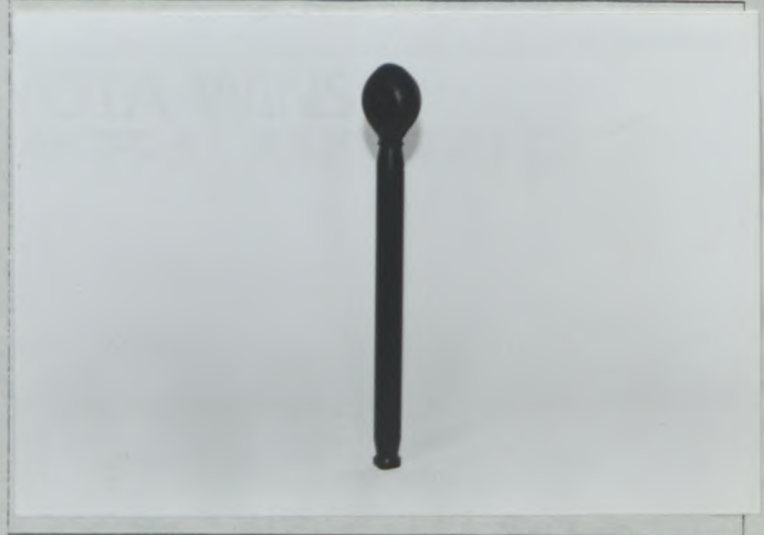
PHOTO 4 : REINFORCED STEERING TRACK ROD
