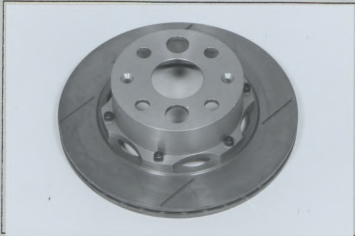
Photo W2 Rear brake disc type 1
