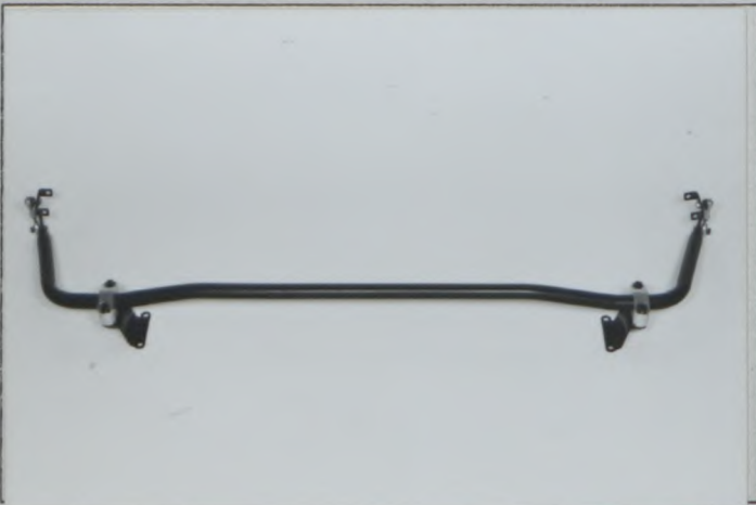
Photo T13 Front anti-roll bar with linkage
