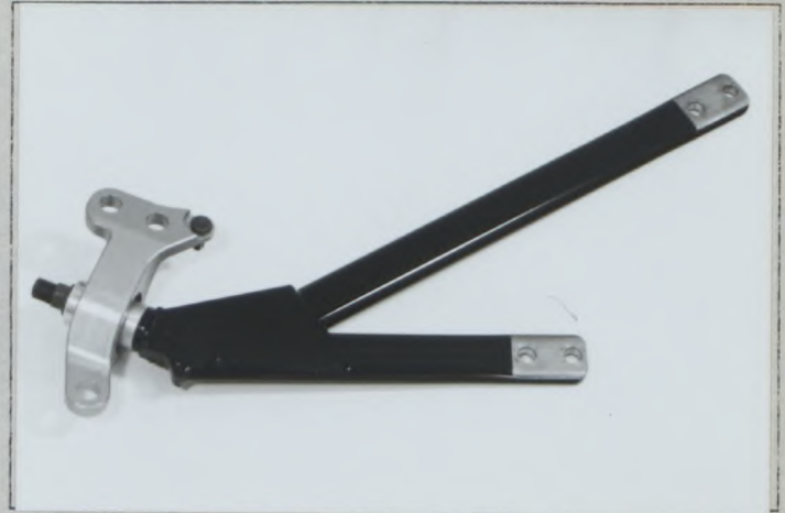
Photo T2 Reinforced front radius arm type2
