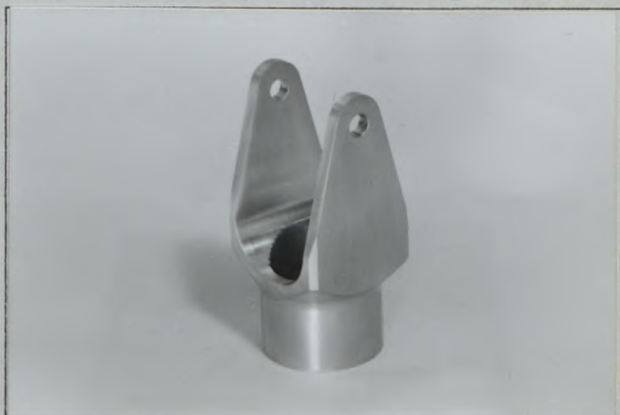
Photo T20 Reinforced rear damper fork
