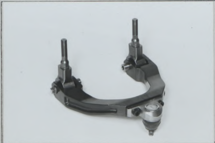
Photo T7 Reinforced front upper arm
