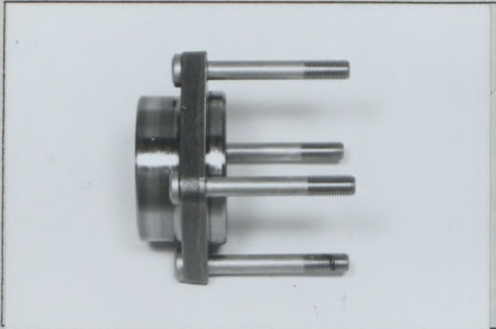
Photo T23 Heavy duty rear hub bearing
