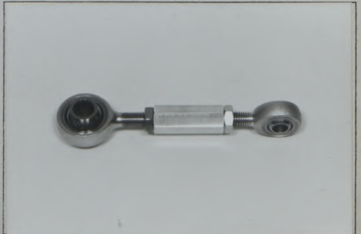
Photo T16 Reinforced rear compensator arm
