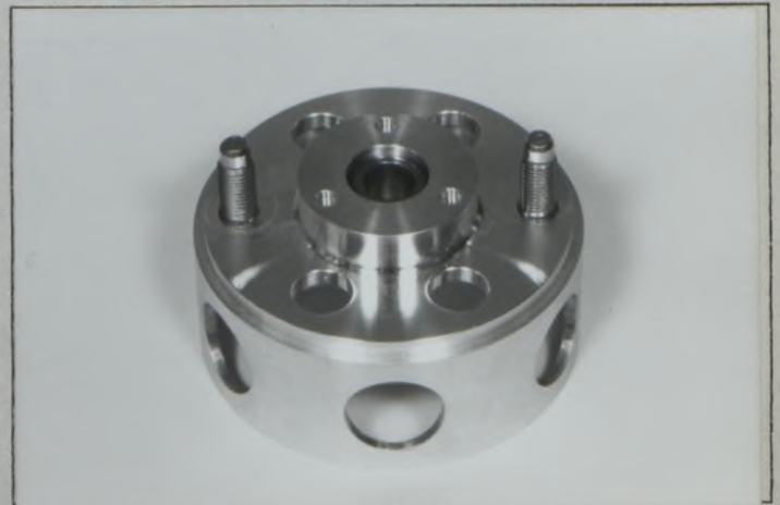
Photo T10 Reinforced front damper mount
