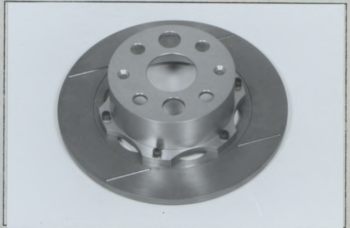
Photo W3 Rear brake disc type 2,3
