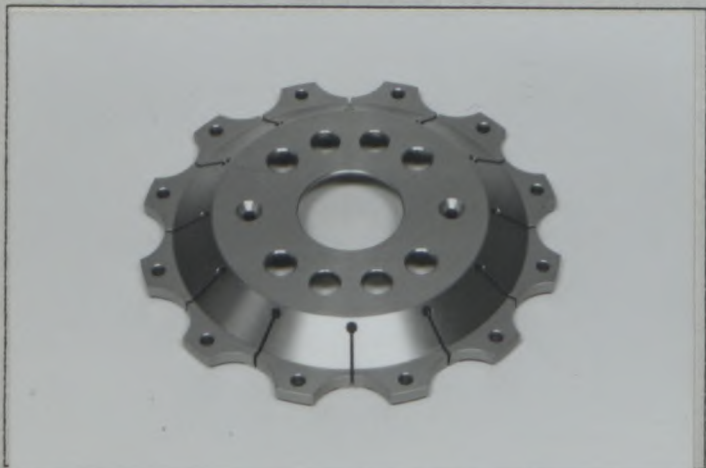
Photo V16 Front mounting bell type 2
