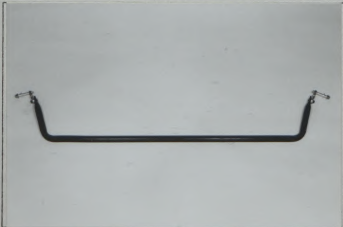
Photo T21 Rear anti-roll bar with linkage
