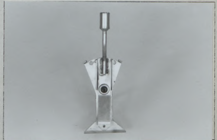
Photo T4 Lever for adjustable rear anti-roll bar
