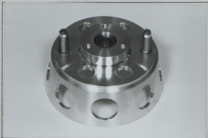
Photo T19 Reinforced rear damper mount
