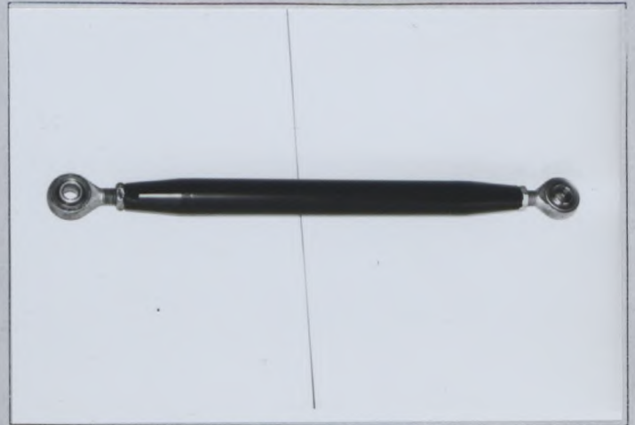
PHOTO U1 REINFORCED LATERAL LINK
