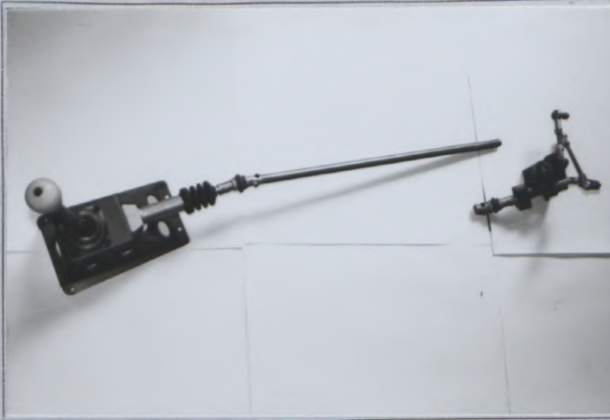
PHOTO S1 REINFORCED GEAR LINKAGE
