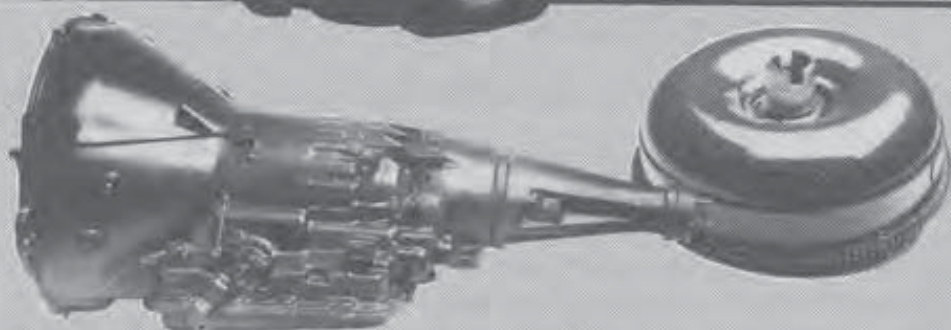
Rod's all-conquering Class 3 truck is equipped with an Art Carr competition off-road transmission, Super Torque converter and heavy-duty shifter.
